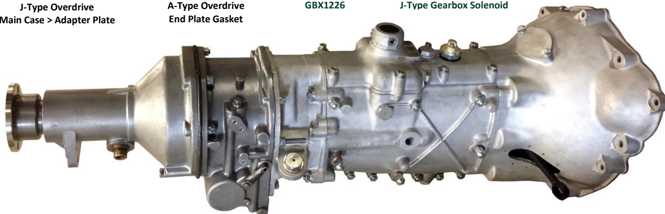
Original 'A Type' Overdrive fitted with short extension unit
