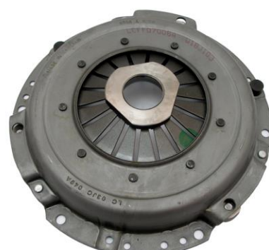
GBX1160 8"/8.5" Diaphragm Clutch Cover (Road) - carbon bearing
