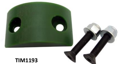
TIM1193 Timing Chain Guide (Fixed) Mounts inside timing cover
